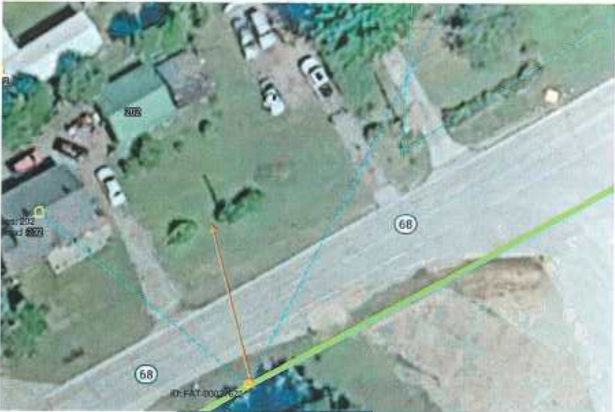
Road shot from MSFN DUCT at 201 W 268 to cross and place Flower Pot in yard of 202 W 68.
